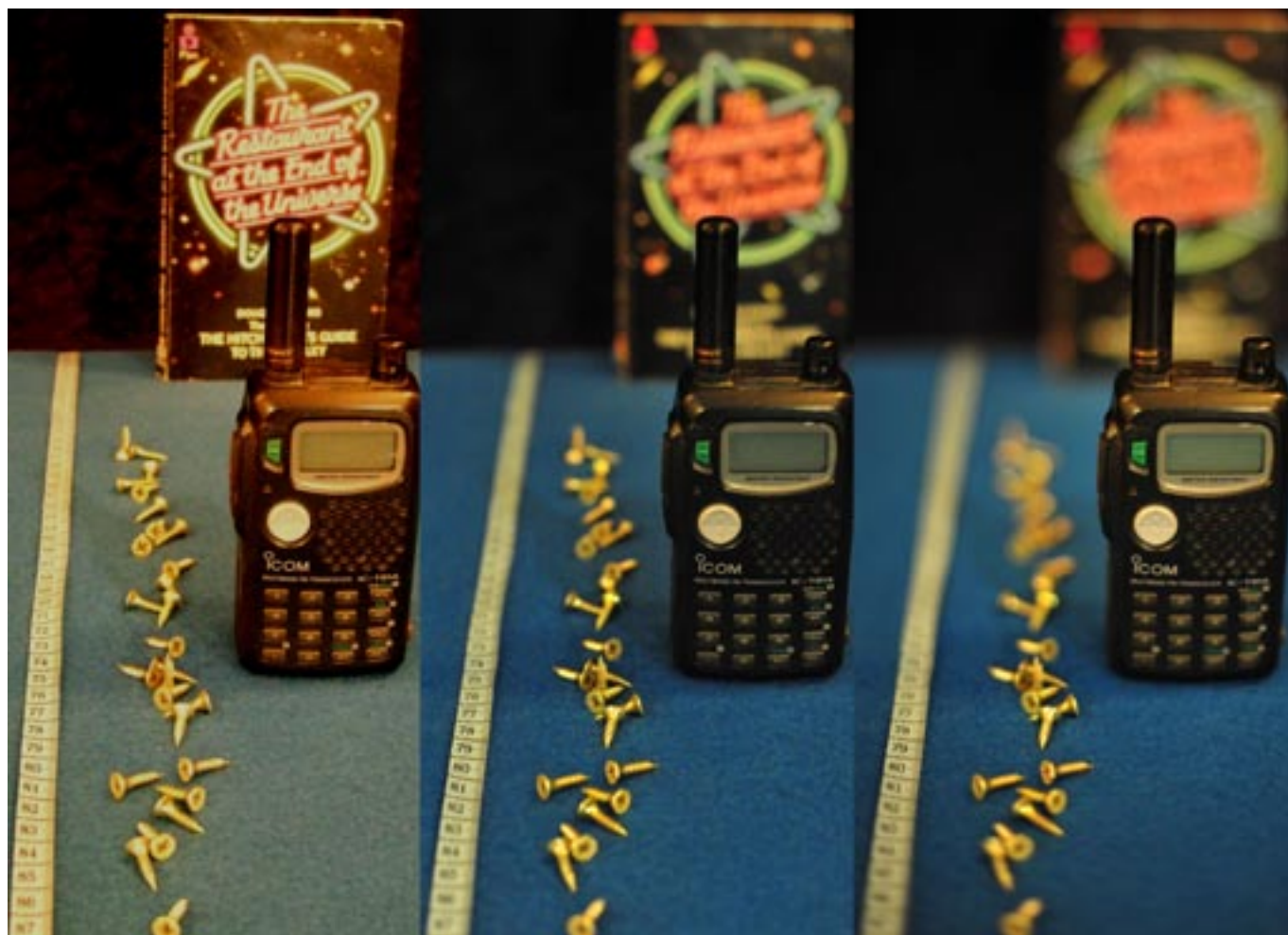
Photo 2 – Same shot, two different cameras. Left: S100FS, 50mm f/3.2. Middle: D700, 50mm f/3.2. Right: D700, 50mm, f/1.4. The book was about 25cm behind the radio. Image: G1MFG
